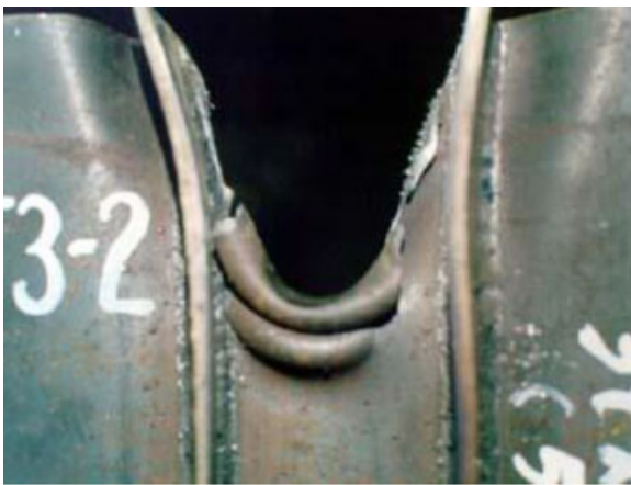
Figure 10.28 A concertina tearing.
